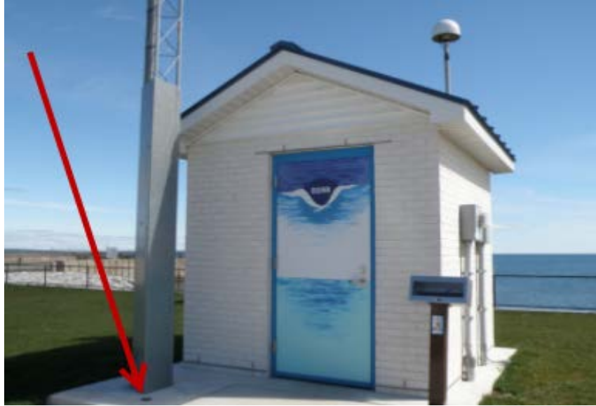
Figure 2.15: An example of a MET SRM consisting of a permanent mark, not a TBM, at the base of a meteorological tower. The mark itself is a bench mark disk at 9075080 Mackinaw City, MI.
