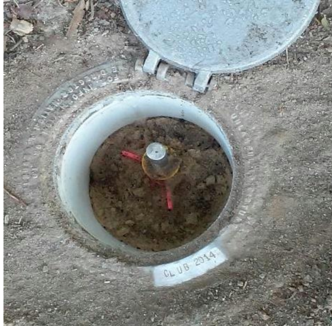
Figure 2.4: Example of a deep rod mark (Class B stability). Logo cap is shown open, to reveal uppermost section of rod mark, greased/finned sleeve, and sand-filled PVC pipe.
