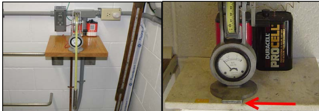
Figure 2.14: On the left is an example of the typical ETG used at a Great Lakes water level station. ETGs are used at all permanent stations in the Great Lakes network as a reference to check the primary and backup water level sensors. The sensor leveling point is shown on the right.
