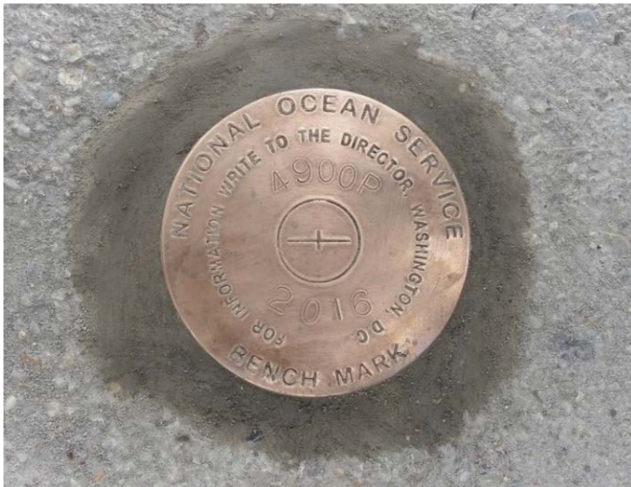
Figure 2.1: Photo of a tidal bench mark disk located at the tidal station 8594900 Washington, DC. Note the organization stamping, National Ocean Service, and the bench mark naming convention, 4900 P 2016.
