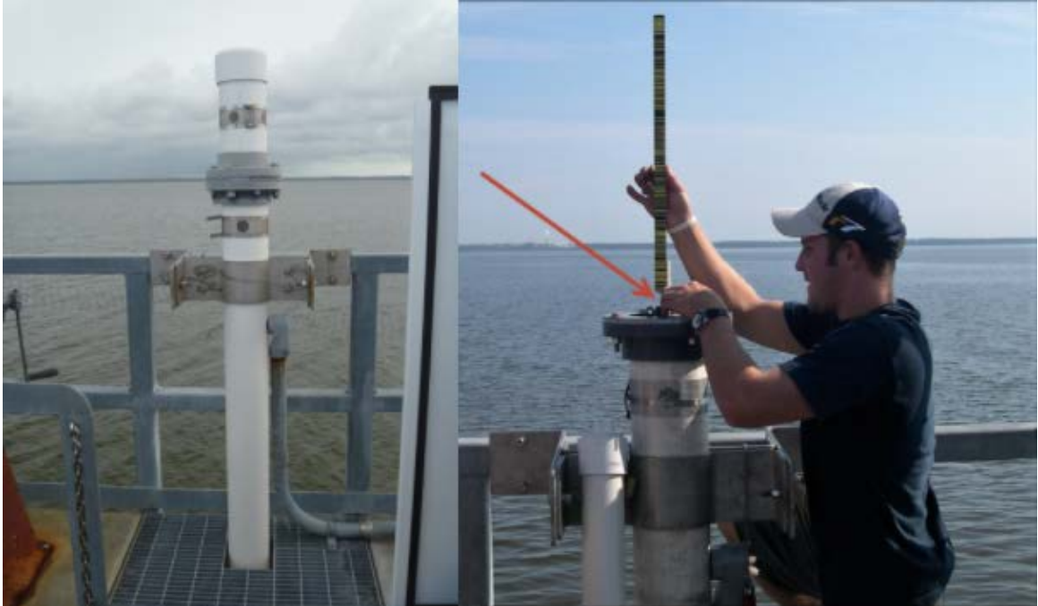
Figure 2.9: The photo depicts an Aquatrak water level sensor and its associated leveling point. In order to access the leveling point, the cap and head must be removed from the sensor setup depicted on the left. After removal, the top edge of the collar should be accessible for leveling.
