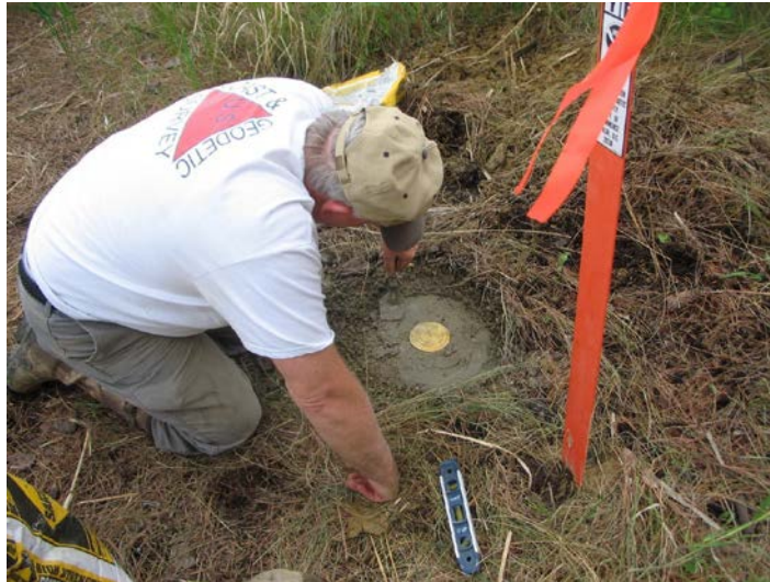
Figure 2.6: Surveyor completing the establishment of a concrete post mark (Class C stability). Note the hand level, which was used to ensure that the top-most surface of the disk was free of obstruction, level to enable successful leveling measurements. Also note the presence of a witness post to assist in mark recovery.
