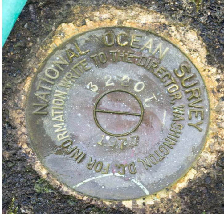
Figure 2.2: The photo depicts an older National Ocean Survey bench mark set for the tidal station 9453220 Yakutat, AK. While originally established in 1977, the format of the stamping is largely identical to present methods.
