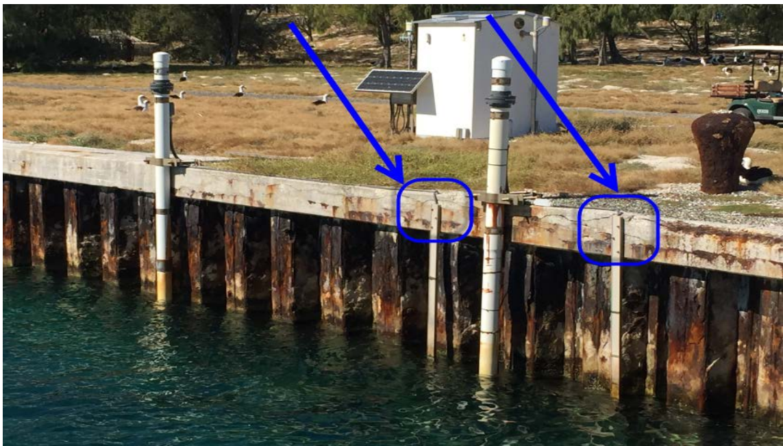
Figure 2.11: The photo depicts a host of water level sensors located at 1619910 Sand Island, Midway. Two ParoScientific pressure sensors are located underwater. The orifice leveling points (circled in blue) are the tops of two wooden boards directly above where the sensors are located.
