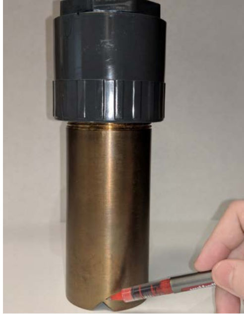
Figure 2.12: The photo depicts a tapedown measurement to a ParoScientific pressure sensor with a V-notch orifice. In this case, the notch is readily visible. However, the amount of growth and biofouling can often make the notch rather difficult to see while in the water. The top vertex of the notch is the leveling point.
