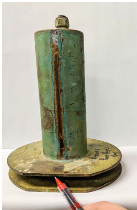
Figure 2.13: The photo depicts a removed parallel plate orifice that would be used with ParoScientific pressure sensor. The bottom of the upper parallel plate is the leveling point of the orifice. As can be seen, the orifices used are subject to corrosion and require inspection.
