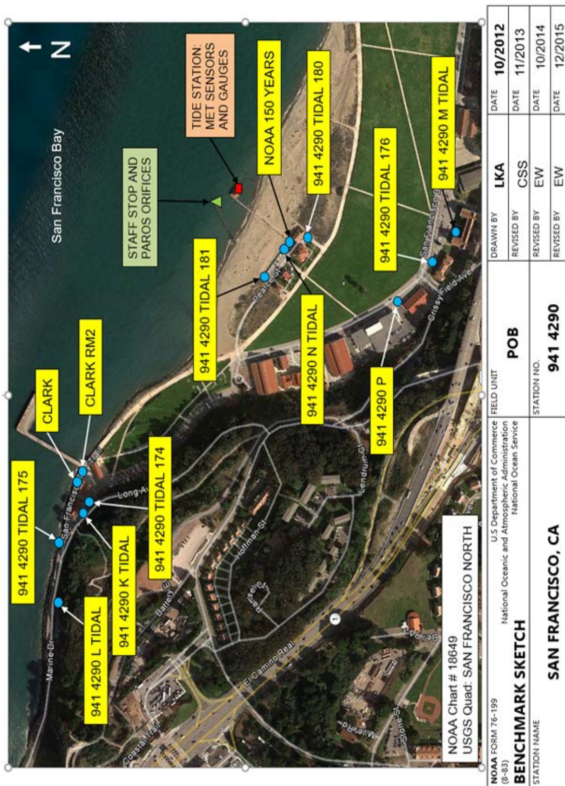
Figure 2.21: Sample bench mark diagram from 9414290 San Francisco provided after an annual inspection to the station. All bench marks associated in the network are listed.
