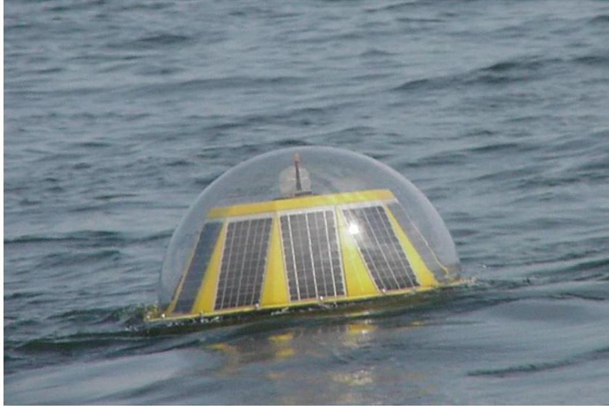
**Figure 4.** TriAxys® Wave Buoy collecting data in waters around Barren Island.
