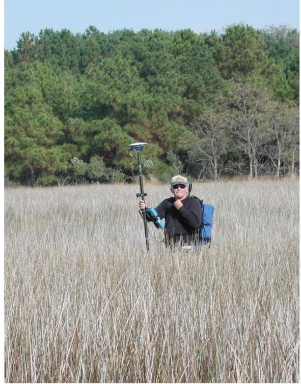
**Figure 8.** Kinematic GPS shows the roving receiver collecting data at various points of interest such as land/water interface, abrupt vegetation change, and geologic features.
