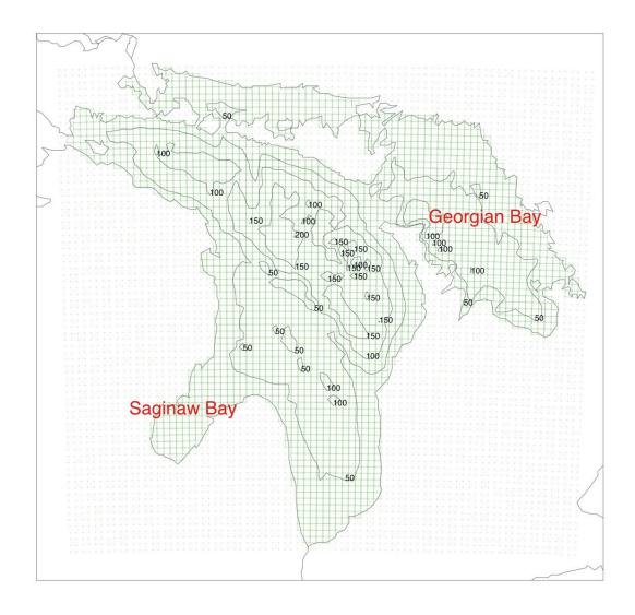
Figure 1. Map depicting the POMGL grid domain (5 km spatial resolution) used by NOS' Lake Huron Operational Forecast System along with model bathymetry contoured at 50 m intervals.
