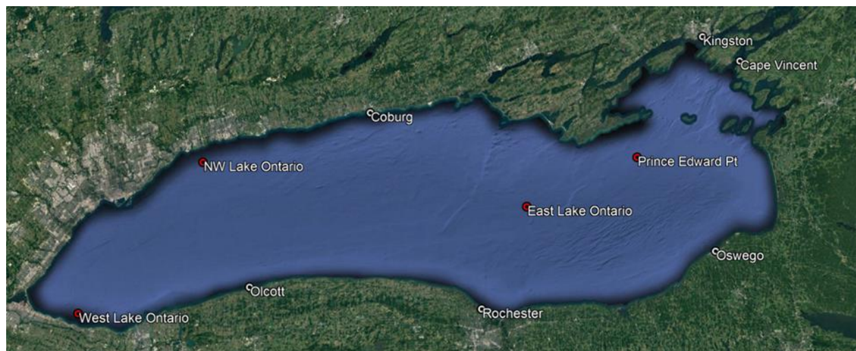
Figure 11. The locations of observation stations used for the Lake Ontario Operational Forecast System (LOOFS) model skill assessment. Water level stations are in white, and water temperature stations are in red.
